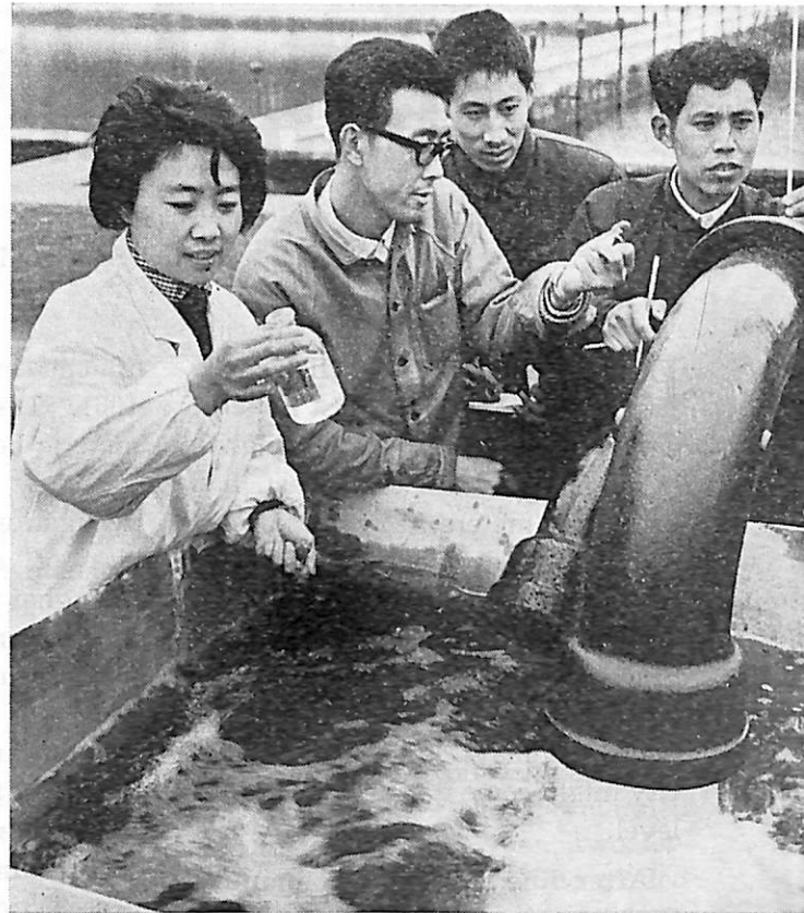
Team members and the water works staff test underground water for purity after surface water has been pumped in to halt sinking.
